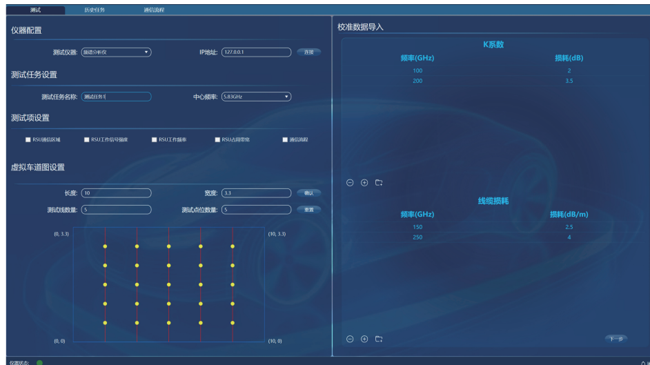
Test Task Configuration Interface: Allows setting up test equipment, test items, and lane-related settings.
