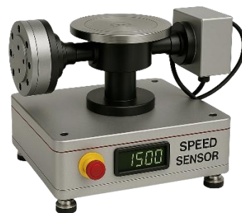
Figure 9: Velocity Sensor Test Bench Schematic
