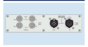
The advanced master clock module AB-AMC processes input and output clock signals to synchronize the audio analyzer with external devices, while generating and analyzing jitter signals for audio analyzers equipped with ADIO, DSIO, PDM, or HDMI modules.
