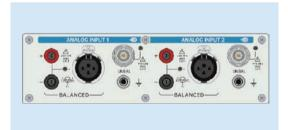
The high-performance analog analyzer option AB-BW52 features ultra-high bandwidth options, providing advanced FFT performance and high-resolution analog input bandwidth of up to 1MHz.
