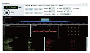
For pure CDR digital signals, the FMH possesses real-time MER testing capability with high MER measurement parameters, fully satisfying transmitter performance testing. Particularly importantly, the FMH can simultaneously test the power of the CDR upper and lower sidebands in real-time.
