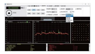
For scenarios where CDR and FM signals are simulcast, general analyzers can only perform spectrum analysis. The FMH features a dedicated filter module, allowing it to continue demodulating the CDR signal and observing channel parameters while performing spectrum analysis. It can also test MER. Despite the strong interference from the FM signal, the FMH can still maximize the demodulation of the constellation
