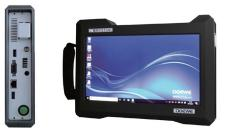
For CDR testing, the FMH can test level/constellation diagram/MER (Modulation Error Ratio), and IQ characteristics. Its high MER testing capability places it directly in the forefront of instruments for transmitter testing, with a comprehensive real-time
