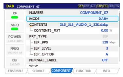
The RWC2010C signal generator supports DAB+ technology, capable of generating high-quality DAB+ signals, helping R&D personnel evaluate the performance of DAB+ systems.
