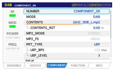
**Encoder:** Converts audio signals into digital format, typically using MPEG-1 Audio Layer II (MP2) encoding, while DAB+ uses the more efficient HE-AAC (High-Efficiency Advanced Audio Coding). The RWC2010C signal generator supports multiple audio encoding formats, including MP2 and HE-AAC, capable of simulating real broadcast environments.
