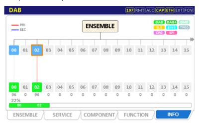
stream, forming an "Ensemble." The RWC2010C's built-in Ensemble Multiplexer supports up to 64 service components for DAB.
