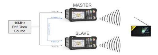
DAB signals are transmitted via wireless broadcast, supporting multiple frequency ranges, typically between 174~240MHz. It employs Single Frequency Network (SFN) technology, allowing multiple transmitter sites to broadcast synchronously on the same channel, effectively saving spectrum resources. Using multiple RWC2010C units can effectively perform SFN testing.
