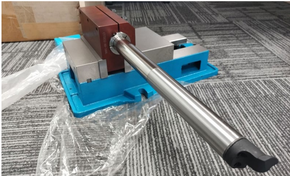
Figure 4 Cutter Fixation Method Display
